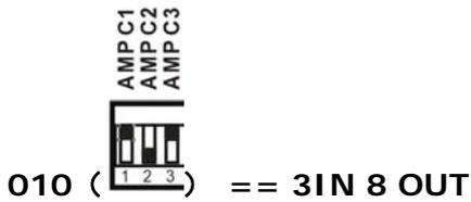
3pcs main amplifier host speaker output connect to AMP port of CH1,CH3 & CH5, audio signal input to CH1&CH3&CH5 input and CH1& CH3& CH5 output to amplifier audio input, First amplifier signal from zone output of CH1,2. Second amplifier signal output from zone output of CH3,4. Third amplifier signal output from zone output of CH5,6,7,8
