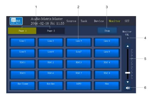
On this monitor screen, you can choose to monitor all the system audio signal. Audio signal includes: the 20bus audio signal(which from master matrix: AUX1-8, SD1, RM1-8, SD2 built-in fire alarm, external timing, external fire alarm), 8 channels zone output audio signal and the wall panel audio input from each zone.
