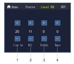
The gain, treble, bass of local audio input can be controlled on this screen.
