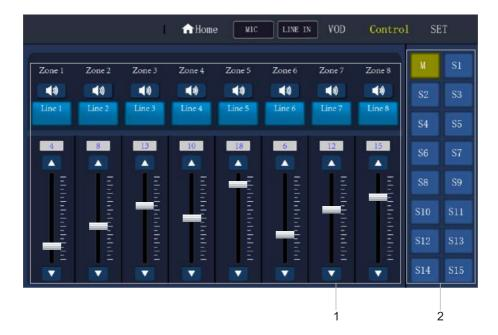
On the control screen, you can see and adjust the volume of every zone, and select the audio source for every zone. It is convenient remote control interface for the operator. It is like operating PA system on the the matrix.
