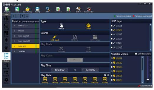
Plan config screen use to set the plan task, the screen includes function buttons, plan list, type, source, play mode, play count, play time, play date, line input of matrix, available zones windows.
