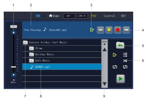
The VOD screen on the microphone station use to play the audio files in the micro SD card. Select the zone first, press talk button to page status, select and play the audio file to related zone.
