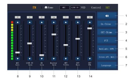
On the set screen, you can set on chime, off chime, PTT, backlight, screen saver time and language. And the audio source (gooseneck microphone, line input, Micro SD) gain, monitor speaker volume, output treble, output bass, output volume can be set here.
